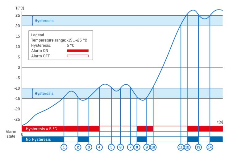
Within the internal 5°C hysteresis band, the alarm would be activated at **point 8** and would end at **point 9**. Because of the hysteresis function, the alarm is extended until the temperature reaches the end of the hysteresis zone (point 10) 5 °C + (-15 °C) = -10 °C.
