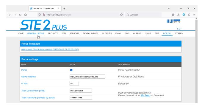
**8.** Team Password can be used in devices to skip the logging procedure during assigning the device to your portal account, or in mobile applications:
