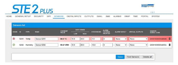
\* Sensor in the Alarm state is highlighted.
