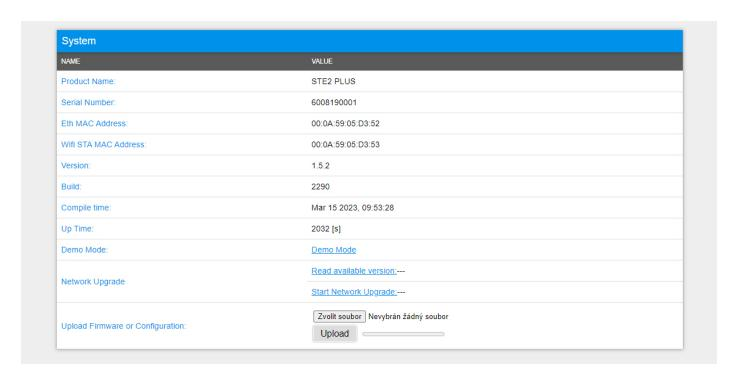
**4) Start Network Upgrade** – Serves to upgrade firmware to the device. The download progress is displayed while upgrading. Click on the Start Network Upgrade link.
