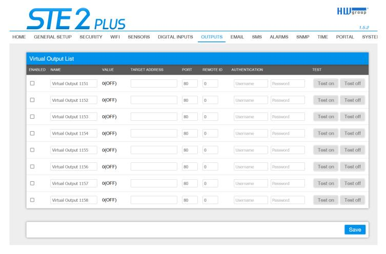
Virtual outputs allow the usage of physical outputs on Poseidon2 or Damocles2 units (Box2Box). VDO (Virtual Digital Outputs) are defined with period (every 60 s).
