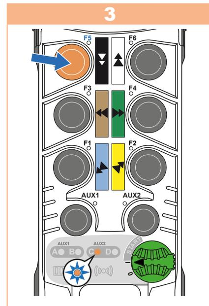
Press the **F5** button to enable the mode:
