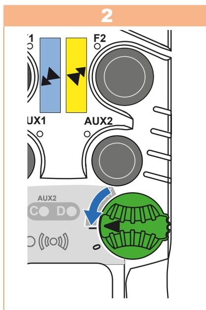
Release the **ON/OFF** switch and all other buttons to start configuration.
