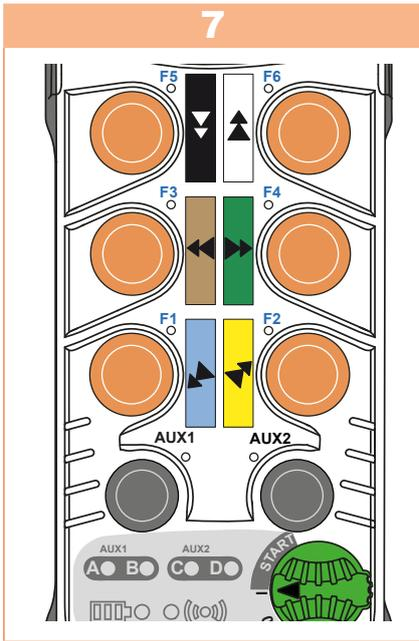
Re-enter the sequence: LEDs A and B go out after each pressing of the **F1 to F6** function buttons. Do not press any button to clear the previous code and disable it at power up.
