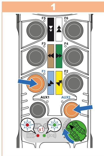
Turn **ON/OFF** switch to the **I** (ON) position. Ensure the LEDs A through D turn on and then off. Then press and hold the **AUX2** and **F1** buttons and turn the **ON/OFF** switch to **START**: Battery and radio LEDs flash once in a loop.
