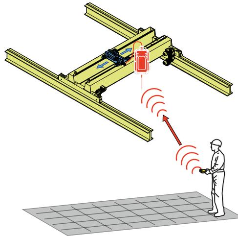
If several devices are equipped with radio controls, working in the same vicinity (e.g., in a factory), each transmitter must carry clear information that tells the operator which equipment it controls. Similarly, the operator must be able to identify the controls corresponding to the directions of movement of the equipment being steered.
