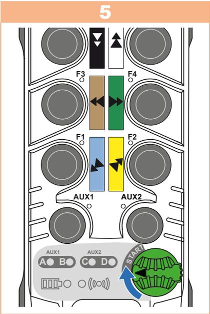
At the end of the sequence, confirm by turning the ON/OFF switch to **START**. **Note:** If the sequence entered is incorrect (length), you are returned to Step 2.
