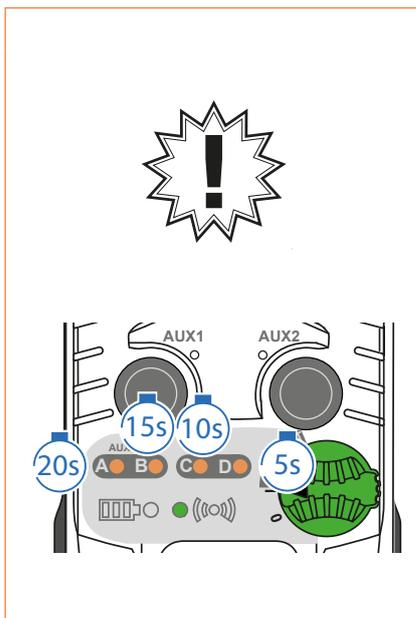
LEDs A, B, C, and D indicate the remaining time by turning off successively every 5 sec in reverse alphabetical order: D after 5 sec, C after 10 sec, B after 15 sec, and A after 20 sec.
