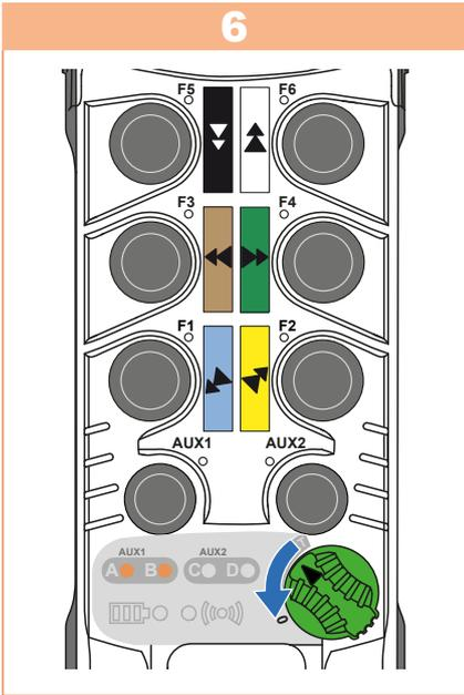
Release the **ON/OFF** switch: LEDs A and B are continuously on to indicate that the code must be re-entered to confirm it.
