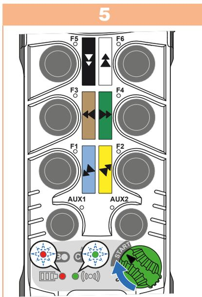
Confirm the value by turning the **ON/OFF** switch to **START**.
