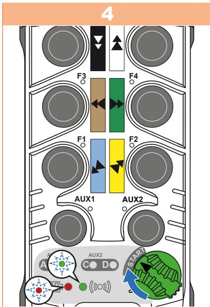
Confirm the value by turning the **ON/OFF** switch to **START**. During transmission:
