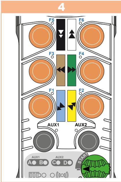
Enter the code by pressing successively on the buttons (chosen sequence): LED A turns off then on after each pressing of the F1 to F6 button. Do not press any button to clear the previous code and disable it at power up.
