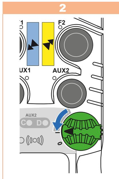
Release the **ON/OFF** switch and all other buttons: LEDs A and B indicate the active release mode (auto or voluntary).
