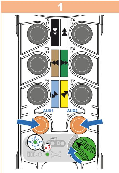
Turn **ON/OFF** switch to the **I** (ON) position. Ensure the LEDs A through D turn on and then off. Then press and hold the **AUX1** and **AUX2** buttons and turn the **ON/OFF** switch to **START**:
