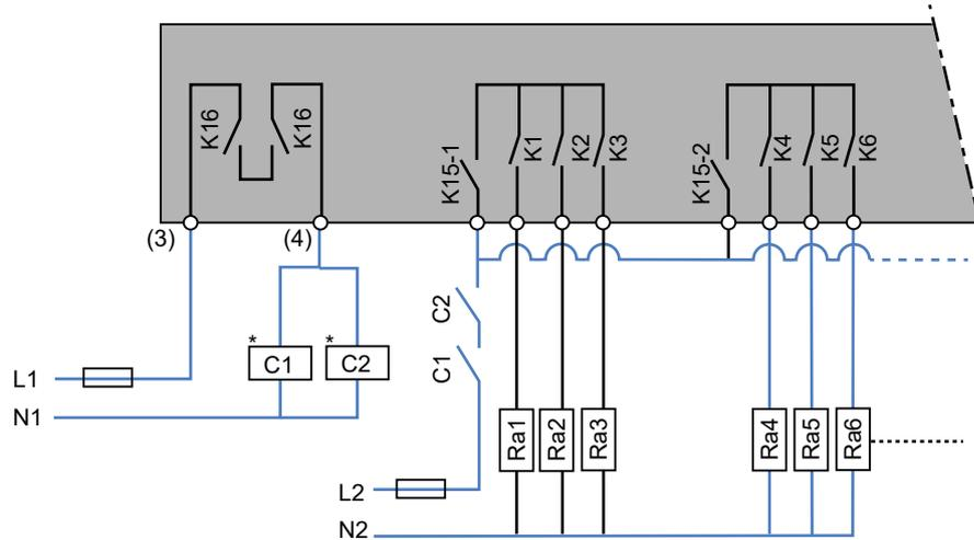
Contactors C1 and C2 are guided contacts, to be integrated in the system safety chain
