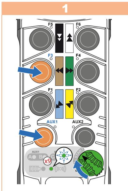
Turn **ON/OFF** switch to the **I** (ON) position. Ensure the LEDs A through D turn on and then off. Then press and hold the **AUX1** and **F3** buttons and turn the **ON/OFF** switch to **START**:
