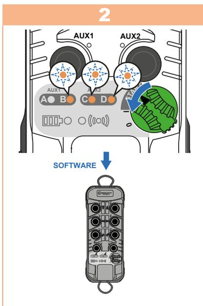
Release the **ON/OFF** switch and all other buttons, the transmitter software version is displayed (green radio LED is off):
