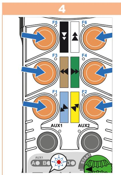
To pre-select a reset press successively the **F1, F2, F3, F4, F5** and **F6** buttons: the battery LED is blinking and all other LEDs are off.
