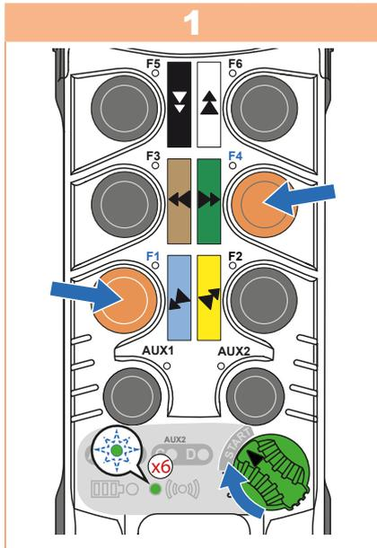
Turn **ON/OFF** switch to the **I** (ON) position. Ensure the LEDs A through D turn on and then off. Then press and hold the **F1** and **F4** buttons and turn the **ON/OFF** switch to **START**:
