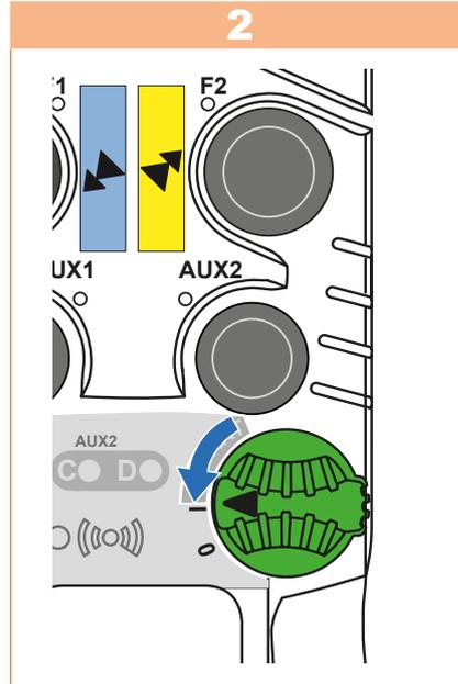
Release the **ON/OFF** switch and all other buttons to start the configuration.
