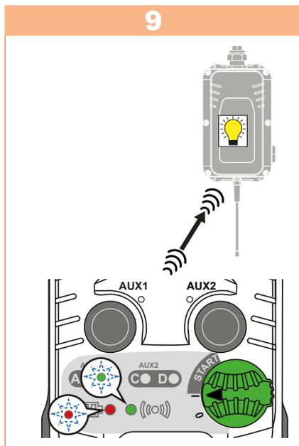
If the two codes entered are the same, the sequence is transmitted to the receiver.
