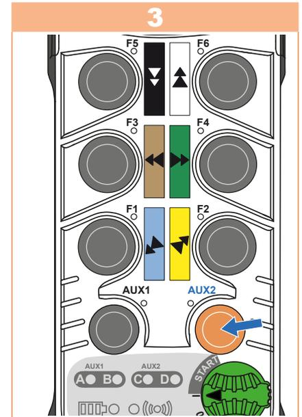
Press the **AUX2** button to enable automatic or manual mode.
