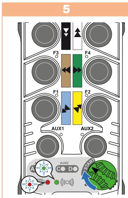
Confirm the channel by turning the **ON/OFF** switch to **START**. During transmission:
