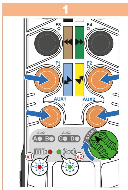
Turn **ON/OFF** switch to the **I** (ON) position. Ensure the LEDs A through D turn on and then off. Then press and hold at the same time **AUX1**, **AUX2**, **F1** and **F2** buttons and turn the **ON/OFF** switch to **START**:
