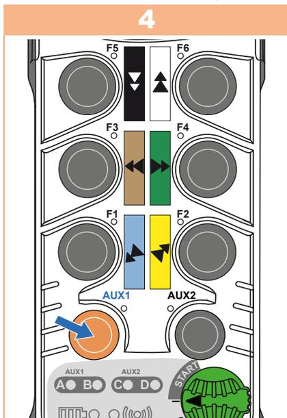
Press the **AUX1** button to scroll the power from 1 to 4.
