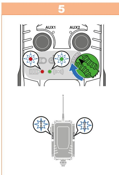
Validate the reset by turning the **ON/OFF** switch to **START**: battery and radio LEDs flash alternately and the receiver memorize the factory defaults (white lamp is on).
