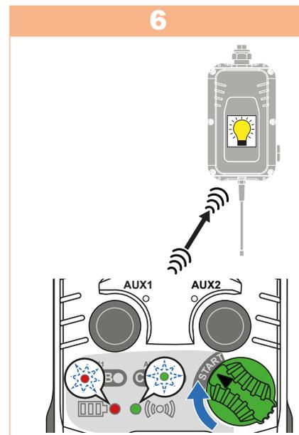
Confirm the value by turning the **ON/OFF** switch to **START**.
