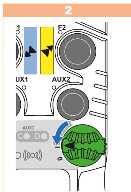
Release the **ON/OFF** switch and all other buttons: LEDs A and B indicate whether the sign of life is enabled or disabled.
