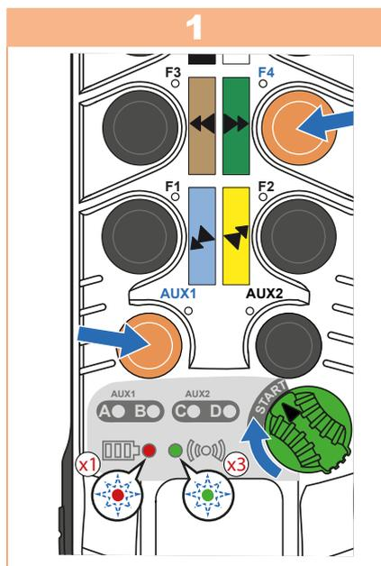
Turn **ON/OFF** switch to the **I** (ON) position. Ensure the LEDs A through D turn on and then off. Then press and hold the **AUX1** and **F4** buttons and turn the **ON/OFF** switch to **START**:
