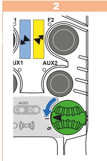
Release the **ON/OFF** switch and all other buttons: LEDs A and B indicate whether swapping is enabled or disabled.
