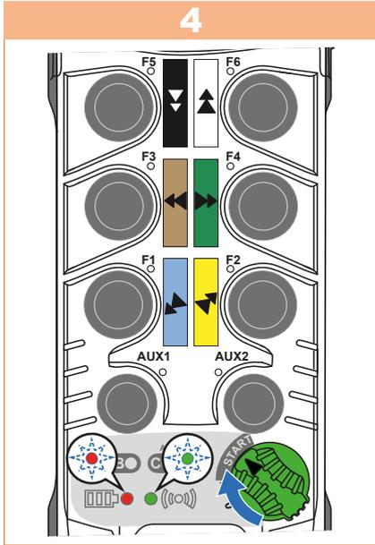
When the desired value is set, confirm it by turning the **ON/OFF** switch to **START**.
