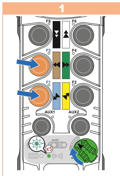
Turn **ON/OFF** switch to the **I** (ON) position. Ensure the LEDs A through D turn on and then off. Then press and hold the **F1** and **F3** buttons and turn the **ON/OFF** switch to **START**:
