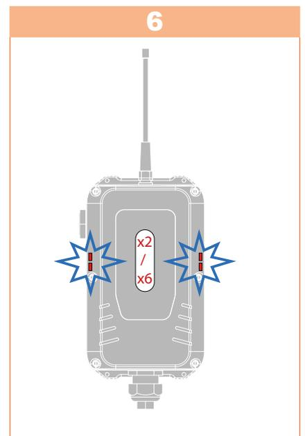
Wait for the receiver's built-in white light to flash quickly: from 2-6 periodic quick flashes.
