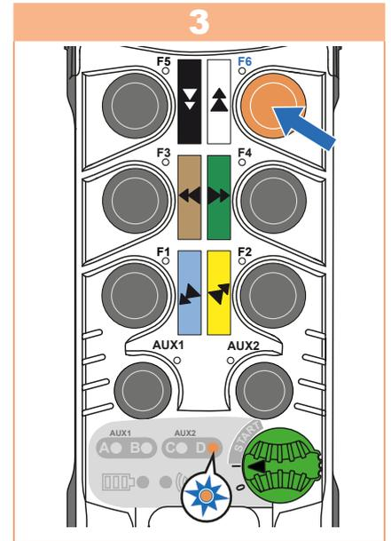
Press the **F6** button to enable the mode: LED D must be on and LED C must be off.
