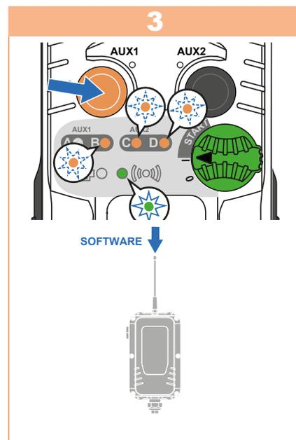
To display receiver software version press the **AUX1** button: the green radio LED turns on and the B, C and D LEDs indicate the version number (in order hundreds, tens and ones).
