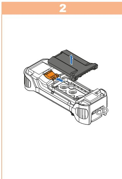
Insert the battery pack into the back of the transmitter.
