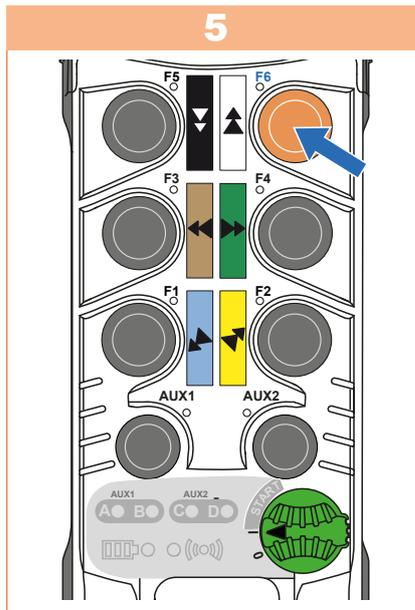
To disable the mode, press the **F6** button. This returns to the fixed radio channel setting (refer to Chapter 8.7.1).
