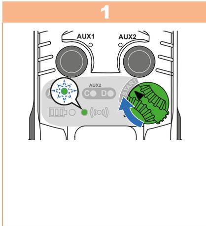
Turn the **ON/OFF** switch to the **I** (ON) position.
