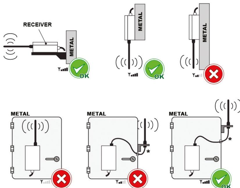
If the installation of the receiver does not allow the operator to see the antenna, it is advisable to offset the receiver antennas under the beams, and point them vertically towards the radio control area, as shown below:
