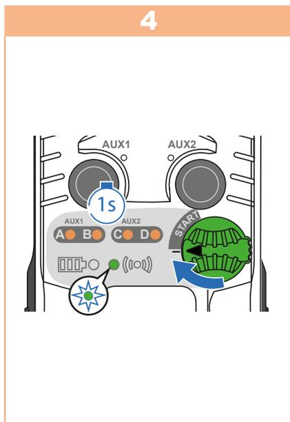
Start the transmitter by turning the **ON/OFF** switch to **I (ON)**<sup>(1)</sup>. LEDs A, B, C, and D light up for 1 sec (initialization phase and self-test).
