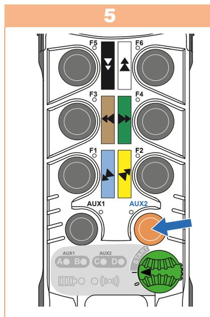
If several receivers have flashing white lights, it is possible to switch from one to the other by pressing the **AUX2** button: the preselected receiver is the one whose light flashes quickly.
