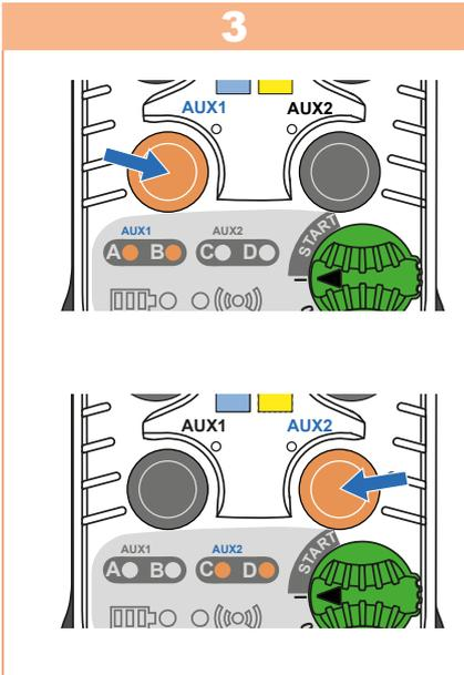
Each time one of the **AUX1** or **AUX2** buttons is pressed, the lighting sequence of the 2 corresponding LEDs indicates the operating mode.
