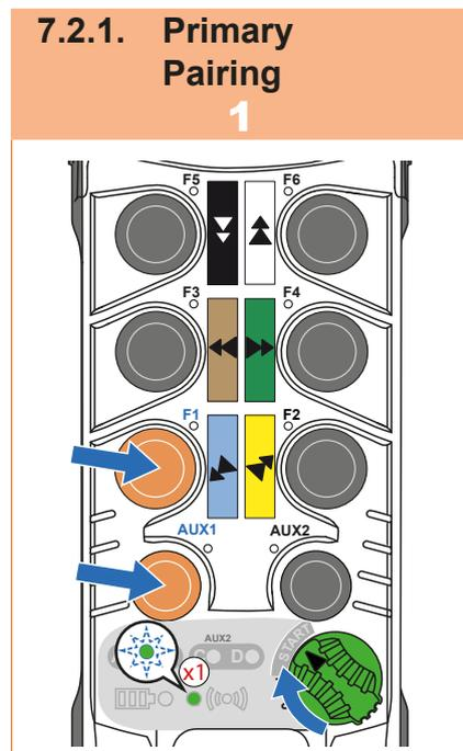
Press and hold the **AUX1** and **F1** buttons and turn the **ON/OFF** switch to **START**:
