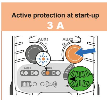
When **LED C** lights on: the protection is active at start-up.
