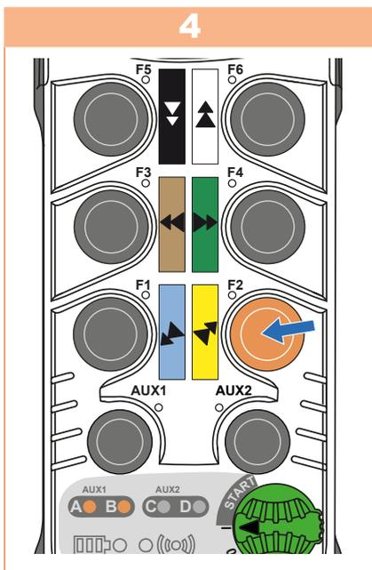
Press **F2** button on the transmitter to stop the scan. LED A indicates the tens and B the ones of the best radio channel found.
