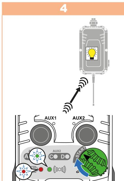
Confirm the selected status by turning the **ON/OFF** switch to **START**. During transmission:
