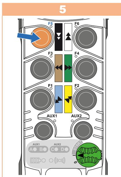
To disable the mode, press the **F5** button. This returns to the fixed radio channel setting (refer to Chapter 8.7.1).
