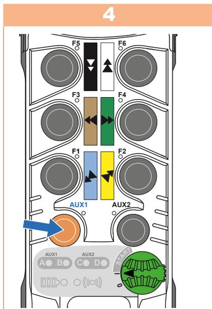
Select the desired sound level using the **AUX1** button.
