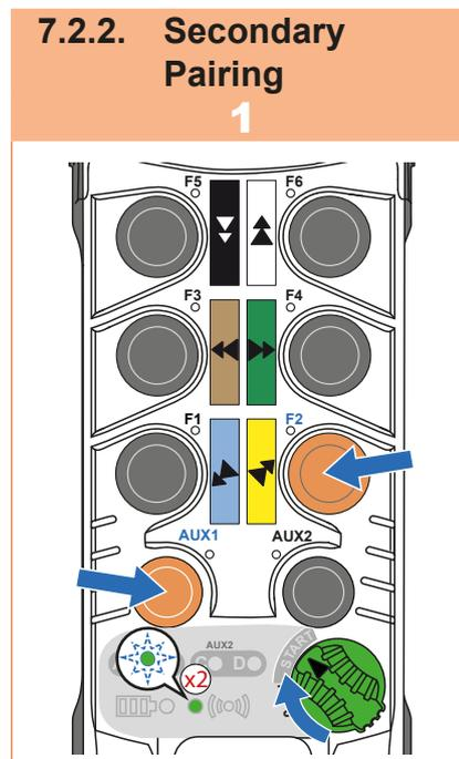
Press and hold the **AUX1** and **F2** buttons and turn the **ON/OFF** switch to **START**:
