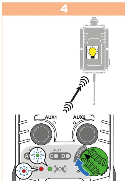
Confirm the value by turning the **ON/OFF** to **START**.
