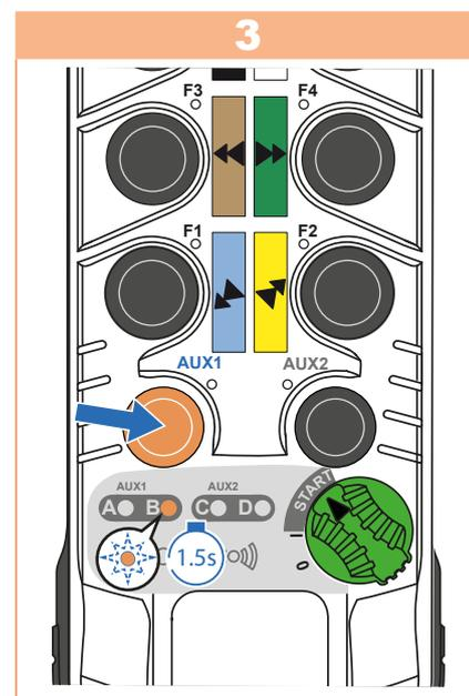
The passive stop delay is factory-set to 0.5 sec and the LED B flashes 2 times.
