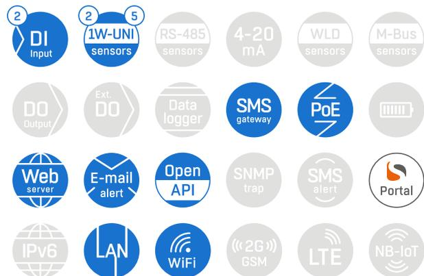
An alert is sent whenever the temperature is too high/low (door is opened). Alerts, such as emails, can be sent directly from the device using SMTP or from the Portal service. Portal also supports SMS, ring-out, and device-invalid alerts.
