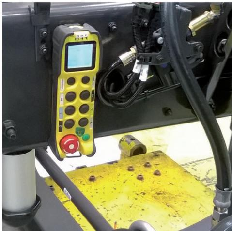
Beta transmitter ready for use on a mobile gear
