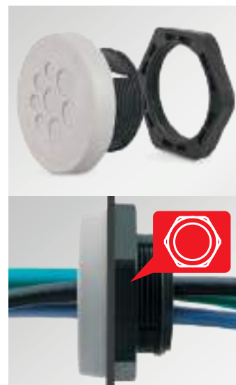
Mounting type 2: Screwed in place with a lock nut For max. wall thickness 11 mm
