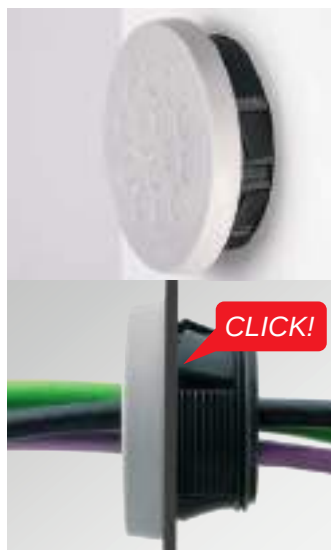
Mounting type 1: Snap into the cut-out For wall thickness 1 – 2.5 mm
