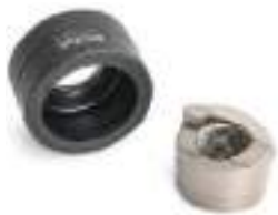
2-fold slug splitting
